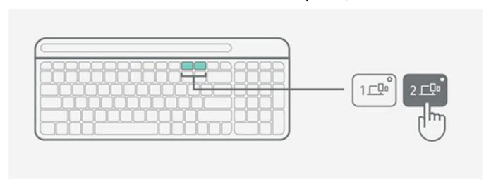
Just click device button on top of function keys for 3 secs.
